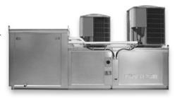
One benefit of this unit is the multiple cooling stages. Multiple cooling stages increase the efficiency by not using 100% of the cooling capacity when this is not needed, thus allowing lower energy usage. An internal make-up air cooling thermostat automatically energizes the first stage when cooling of the make-up air is required. The same thermostat has a built in adjustable differential to energize the second stage of cooling when required.
